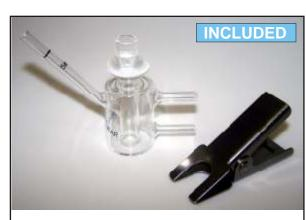
This diffusion cell is the most common Franz Cells. It is a jacketed Franz Cell with 9mm orifice diamter, flat ground joint, and 5ml receptor volume. It is the defacto standard for working with human skin and may be used with any membrane4mm or less thickness.
